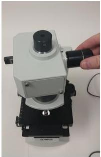
The camera port is located on the opposite side of the view mode switch
