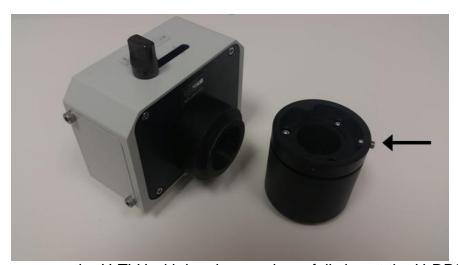
Loosen set screw on the U-TLU with hex key, and carefully insert the U-DPCAD. Once inserted, tighten set screw to secure U-DPCAD.
