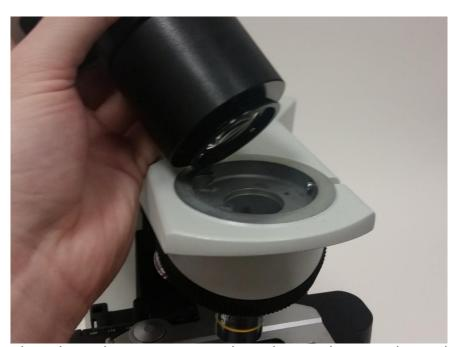
Carefully place the entire upper mount where the eyepiece was located. Use the eyepiece set screw on the right side of the arm to secure the upper mount in place.
