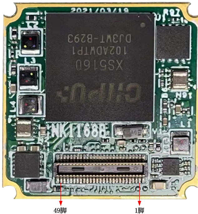
Fig. 2-1 The coordinate diagram and the entity of HRS 50-PIN interface
