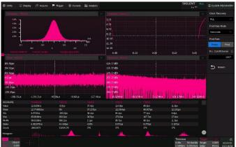
Supports eye diagram and jitter analysis/measurement. It can automatically extract the embedded reference clock from serial data and create the eye diagram. Measurement on multiple eye/jitter parameters is provided. Mask test on eye diagrams is supported
