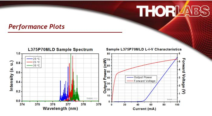
This data will vary for each diode. The sample spectrum of the L375P70MLD laser diode was taken at 20 °C, 25 °C, and 30 °C. The measurements were taken using a Thorlabs OSA201 Spectrum Analyzer. The L-I-V data was taken at 25 °C.
