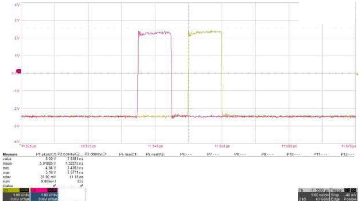
Figure 3: Oscilloscope screen capture, generation of two narrow pulses (5 ns) with 7.5 ns of Delay(s) one from the other.
