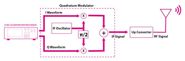
Figure 7: AWG for Baseband signals (TX) - Arb Rider AWG-506X
