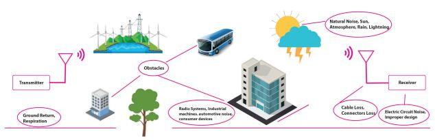
Figure 1: Wireless Data Transmission - Noise and Loss may cause Errors -
