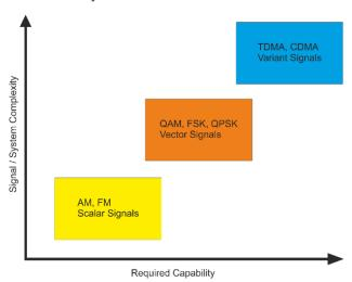
Figure 2: Analog & Digital Modulations
