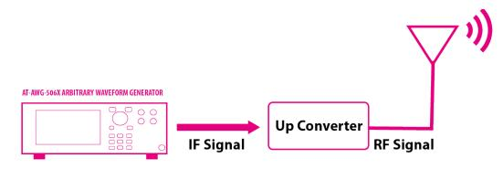
Figure 9: AWG for IF signals (TX) - Arb Rider AWG-506X
