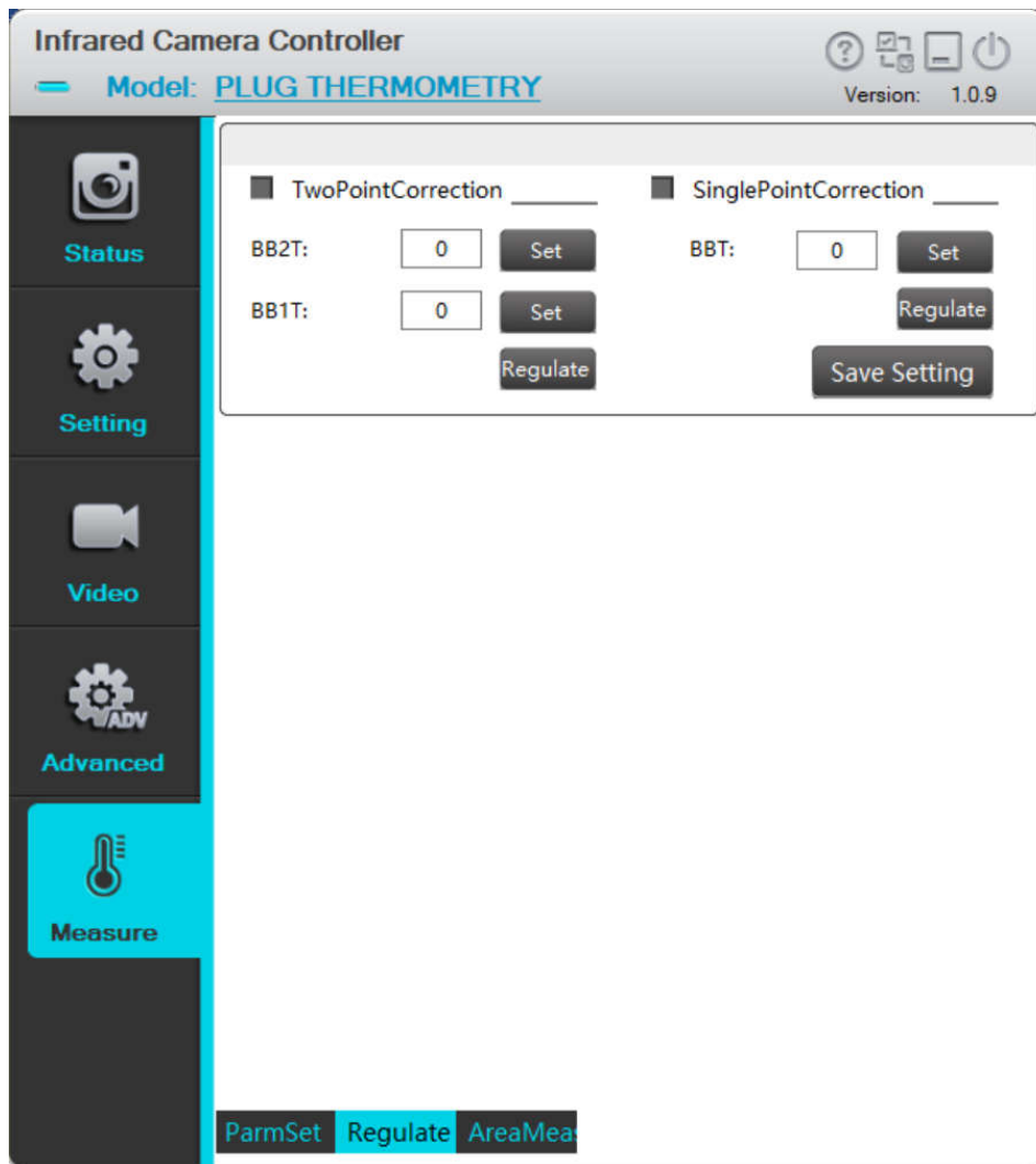
Fig.4-31 blackbody correction interface
