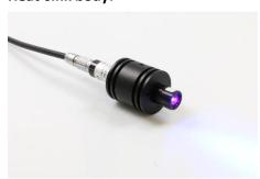
The heat sink allows the UFIBER to produce a more powerful light by improving the heat management.
