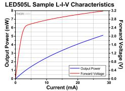
These measurements were taken at a case temperature of 25 °C. The output spectrum and radiation distribution were measured with an operating current of 20 mA.
