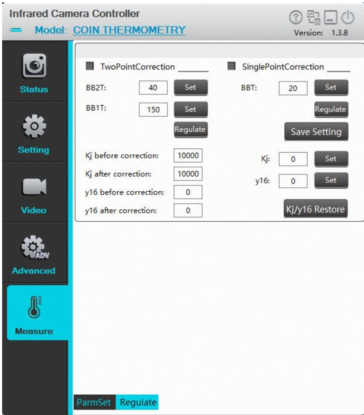
Fig.4-33 blackbody correction interface
